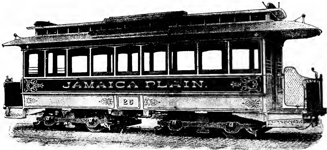
Fig. 5646. CLOSED ELECTRIC-MOTOR CAR. WEST END STREET RAILWAY, BOSTON. BUILT BY J. M. JONES' SONS, WEST TROY, N. Y. Equipped with Bemis Four-wheeled Trucks.
